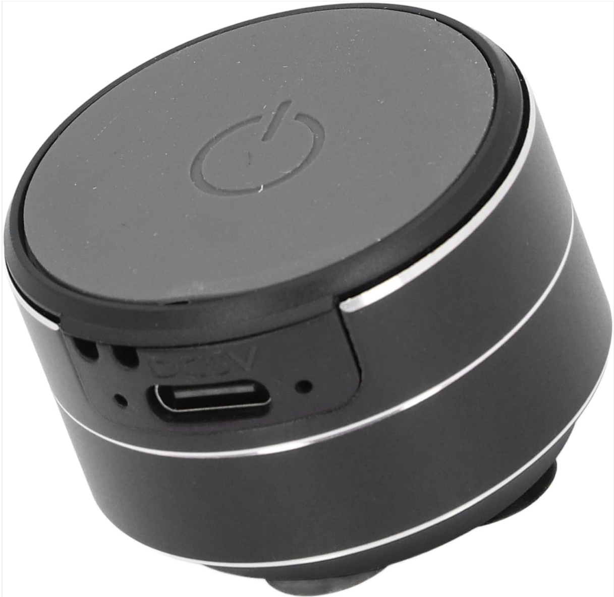
Image 4.1: Close-up of the speaker's side, indicating the USB charging port.
