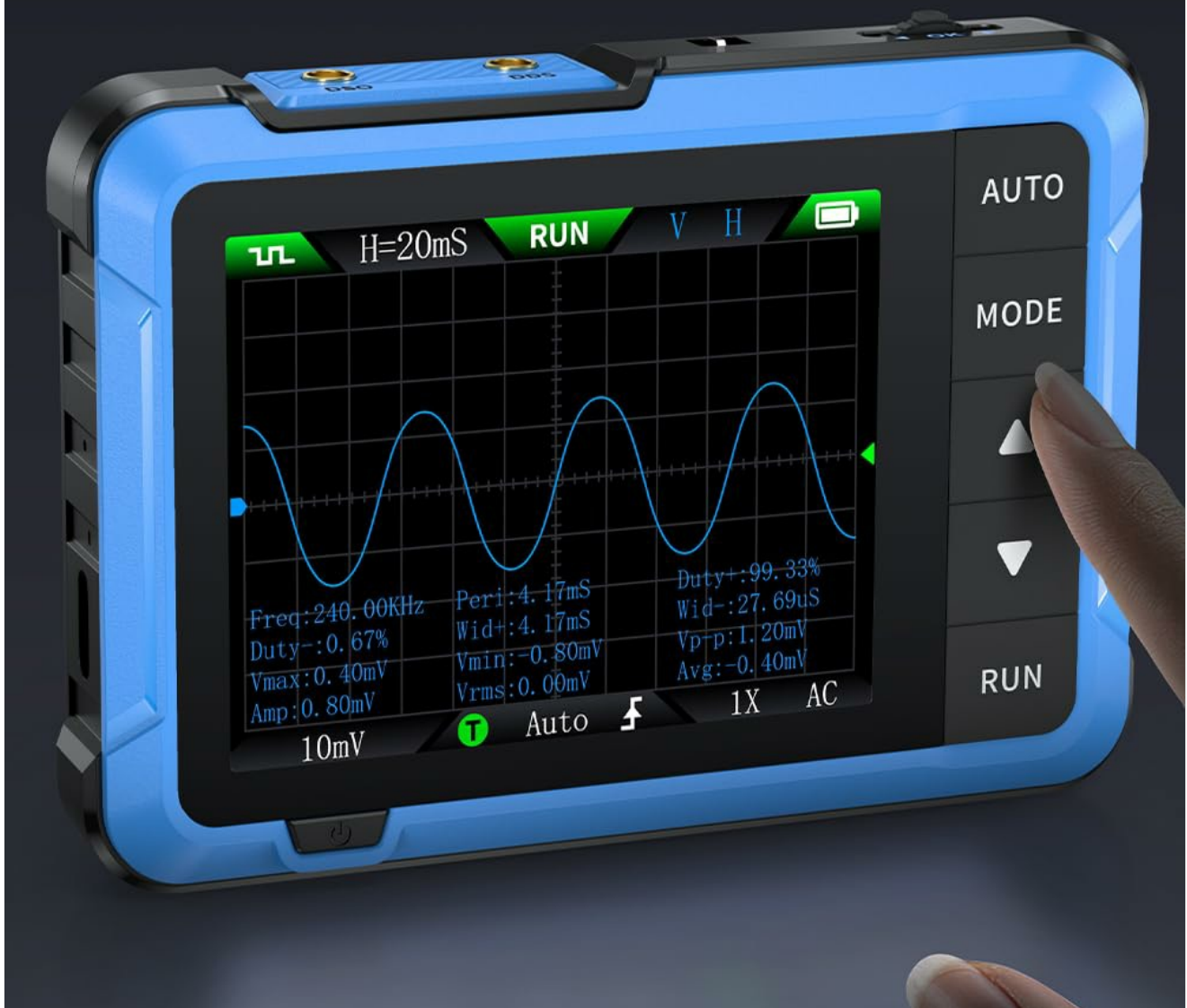
Figure 4.3: User interacting with the DSO-510 to analyze a waveform, highlighting the device's support for waveform pause, zoom, and movement for detailed insights.
