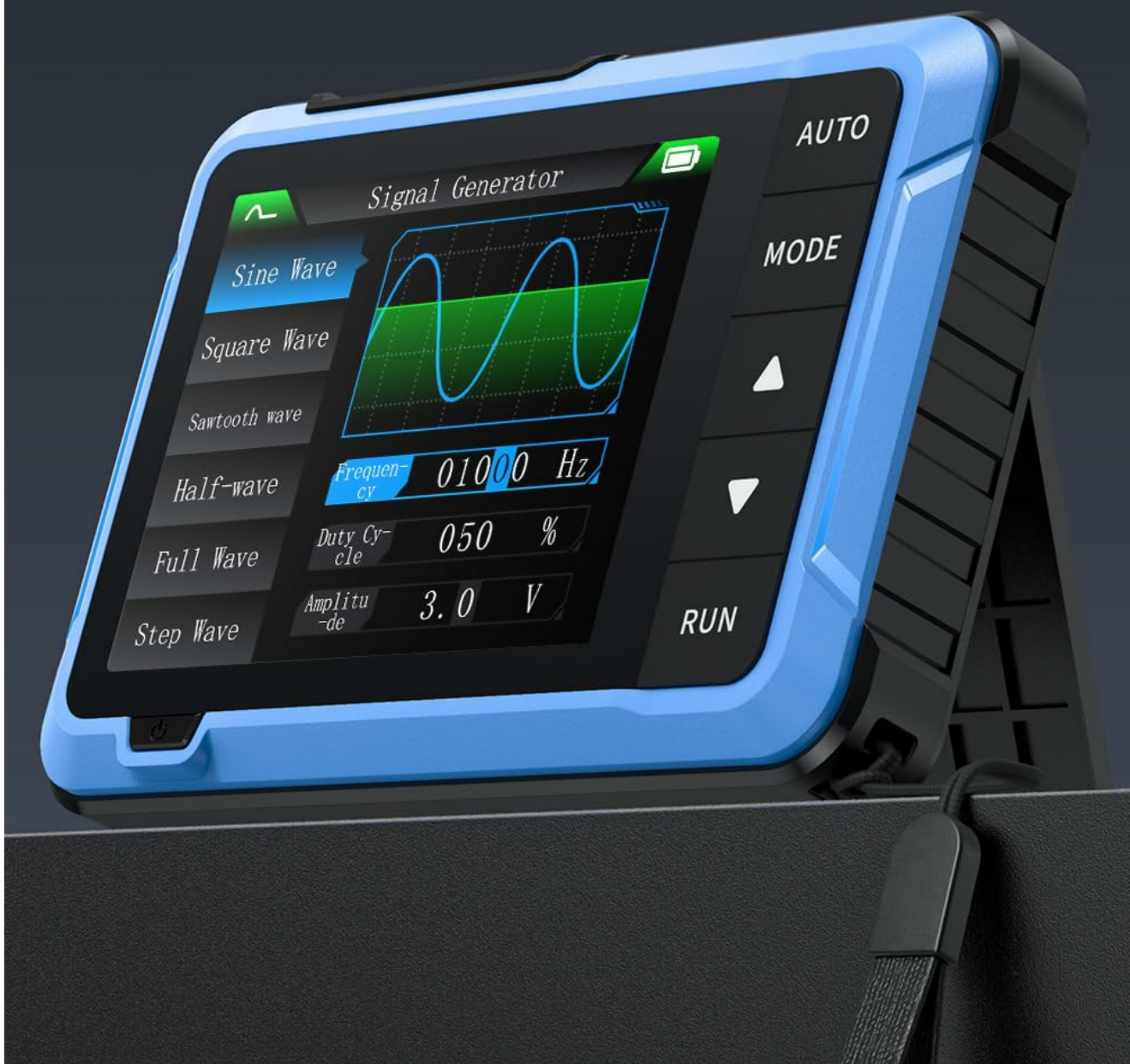
Figure 4.4: The DSO-510 in Signal Generator mode, showing options for selecting waveform types and adjusting frequency, duty cycle, and amplitude.
