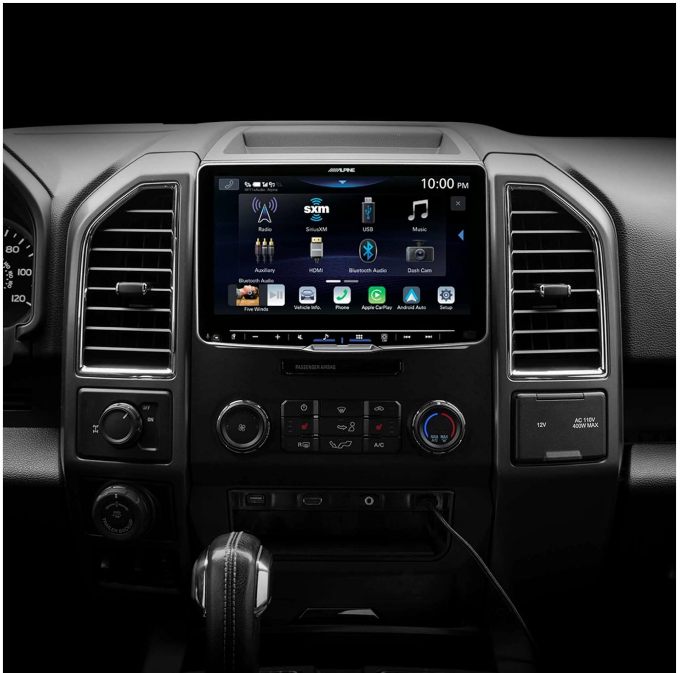
Image 5.1: The main menu screen of the Alpine Halo9 ILX-F509. This interface provides access to various functions such as Radio, SiriusXM, USB, Music, Auxiliary, HDMI, Bluetooth Audio, Dash Cam, Vehicle Info, Phone, Apple CarPlay, Android Auto, and Setup.
