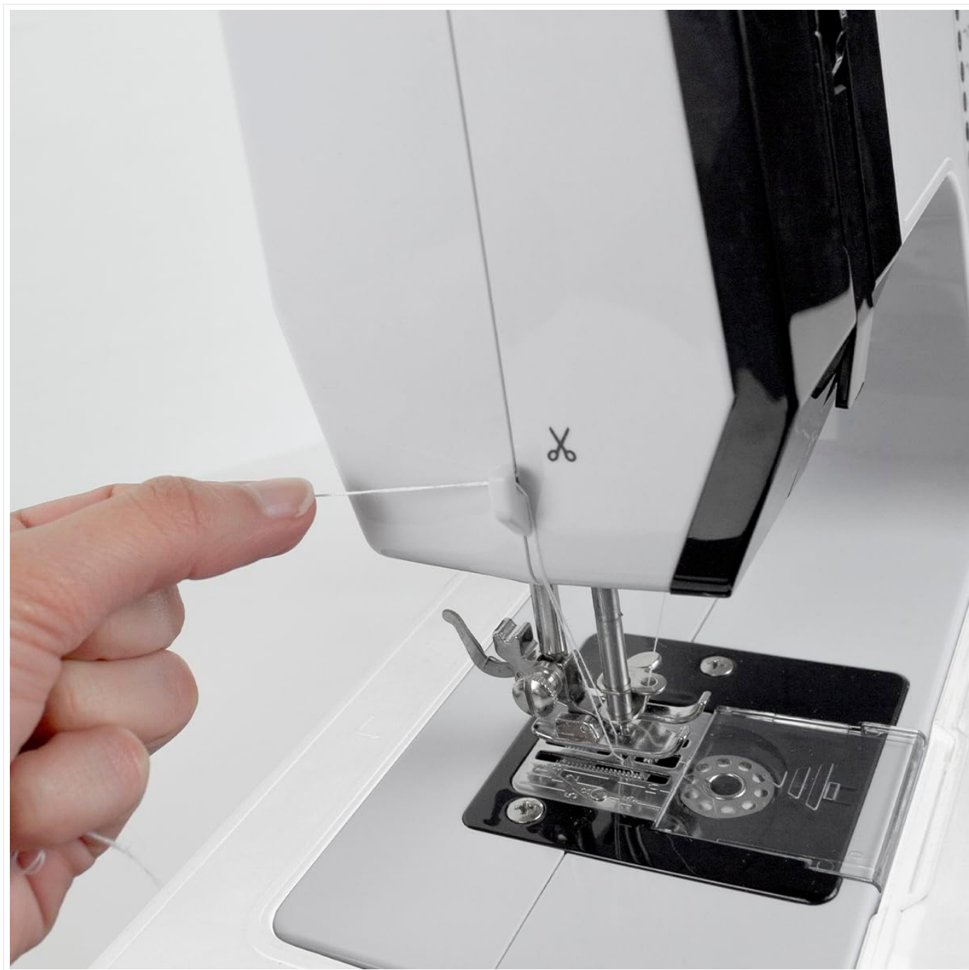
Image: A close-up of the integrated thread cutter on the PRIXTON P125 sewing machine.
