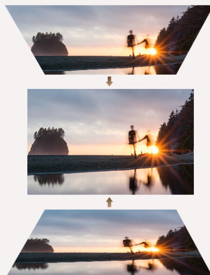
Figure 5: Illustration of auto vertical keystone correction and manual focus for optimal image display.
