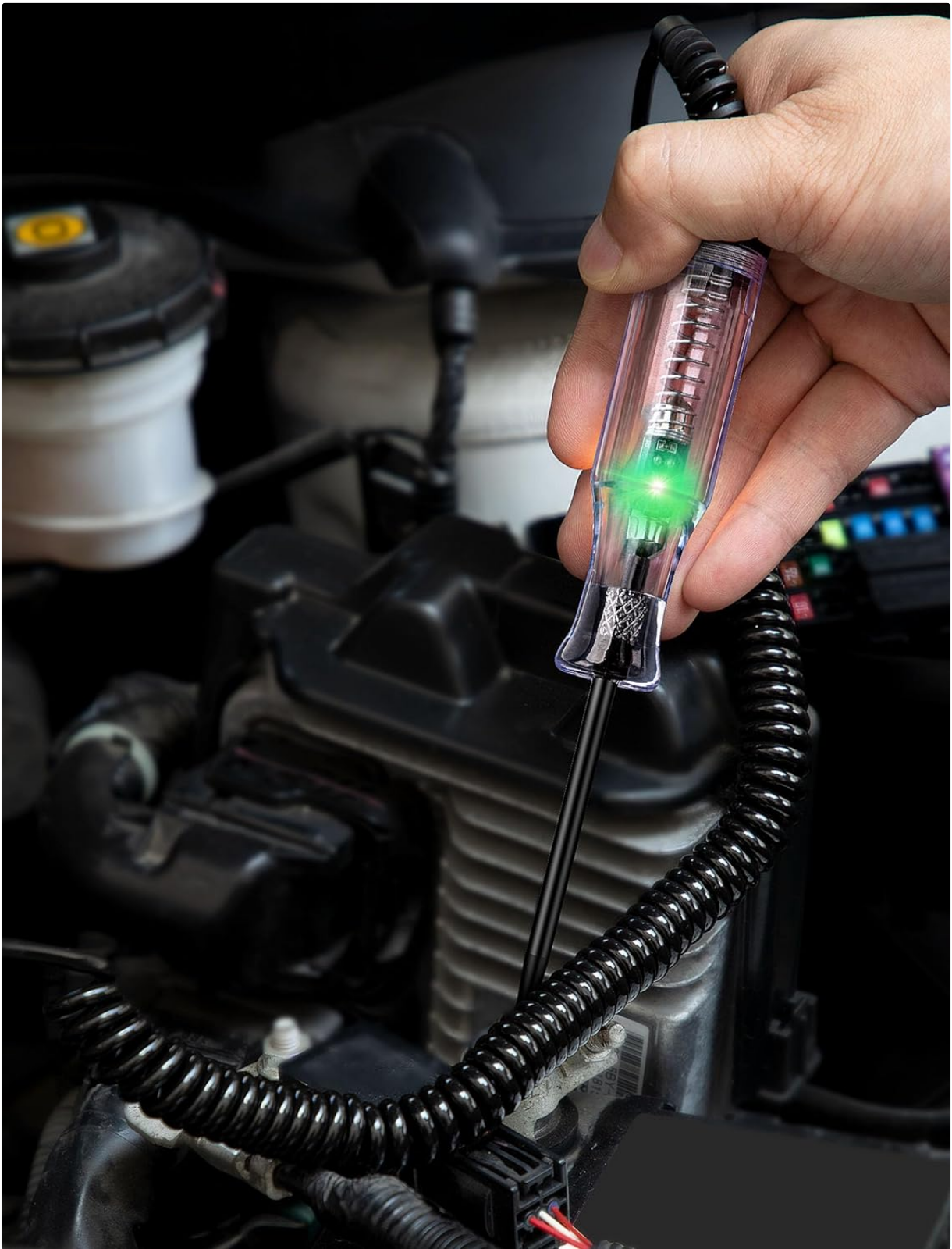
Image 4.1: The circuit tester being used on a vehicle's electrical system, showing a green light indicating negative polarity.
