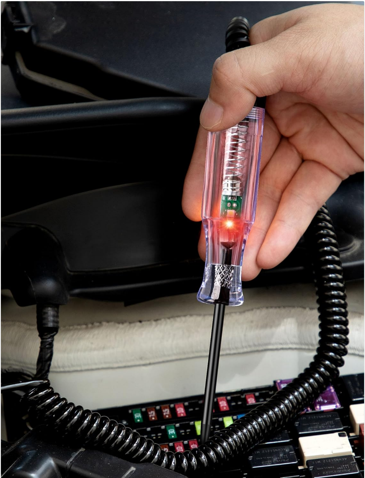
Image 4.2: The circuit tester being used on a vehicle's electrical system, showing a red light indicating positive polarity.
