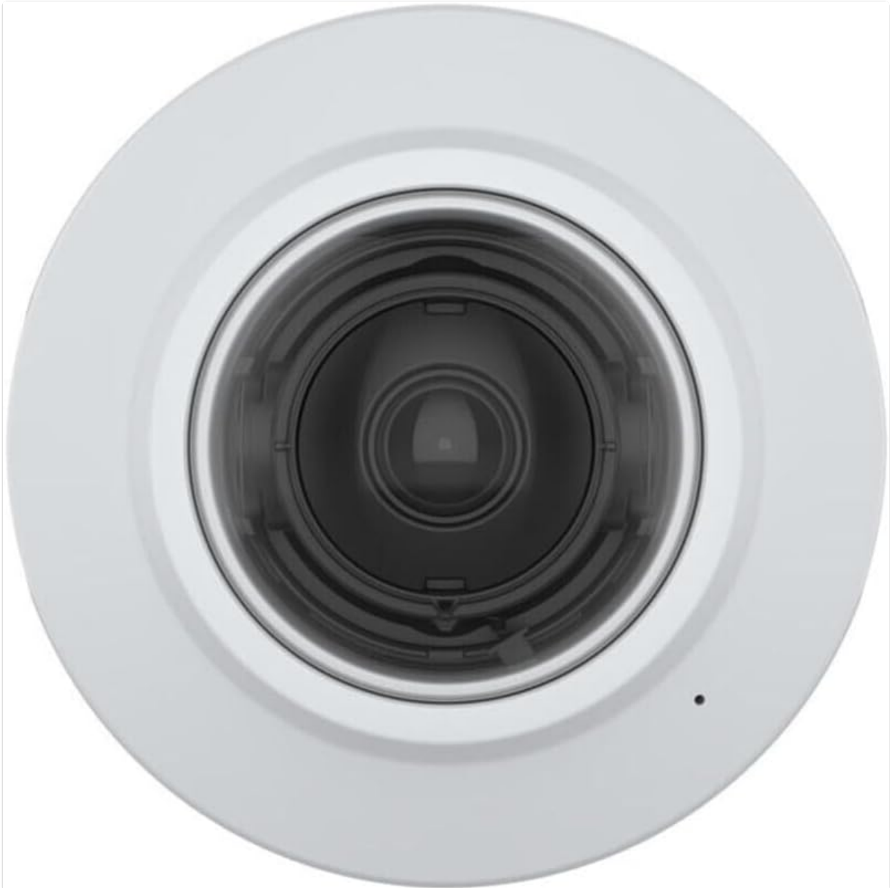
Figure 5.1: Top-down view of the Axis M30 Series M3086-V camera, showing the central lens and surrounding casing.
