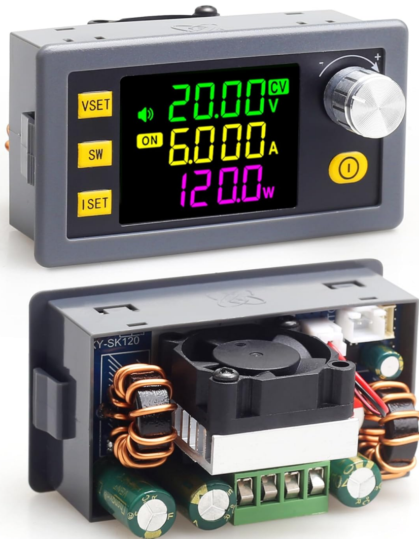
Figure 1: Front and internal view of the SK-120 Buck Boost Power Converter, showcasing its display and internal components.
