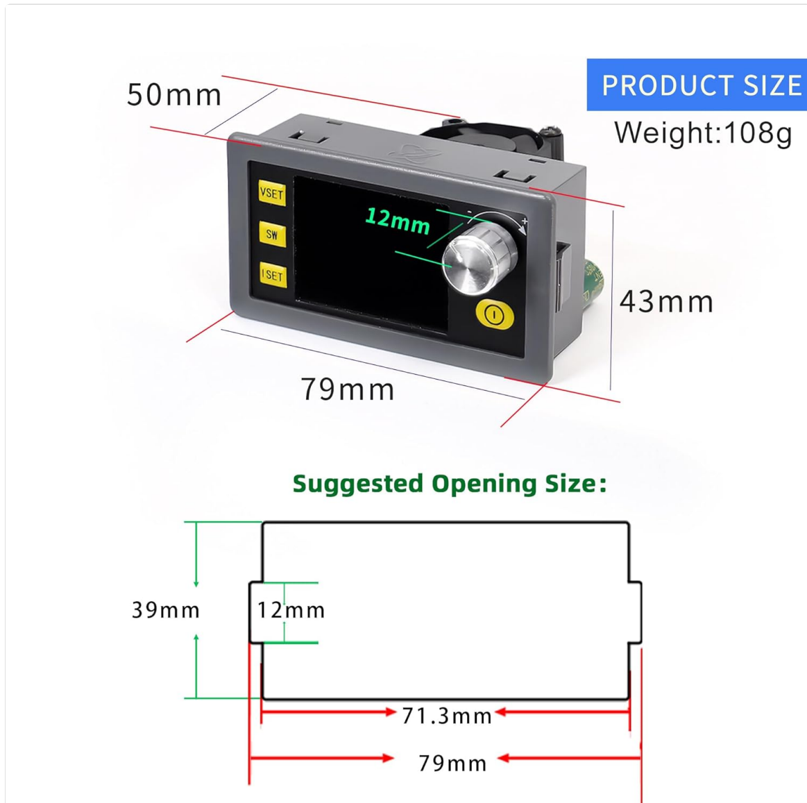
Figure 5: Dimensions of the SK-120 module and recommended panel opening size for installation.
