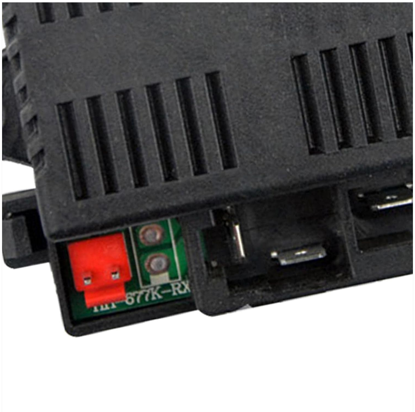
Image 2.2: Close-up view of the connection ports on the HH678K-2.4G receiver, highlighting the wiring interface and control board.
