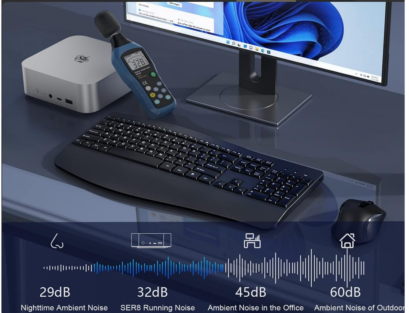
Figure 3.9: Quiet Operation. This image illustrates the low decibel, ultra-quiet operation of the Beelink SER8, showing its running noise at 32dB compared to nighttime ambient noise (29dB), office ambient noise (45dB), and outdoor ambient noise (60dB).
