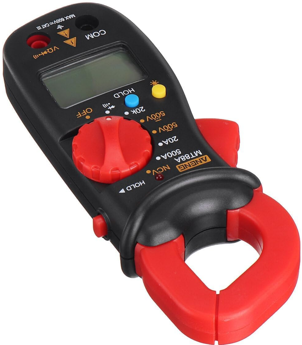
Figure 4.2: The 'HOLD' button, used to freeze the current measurement on the display.
