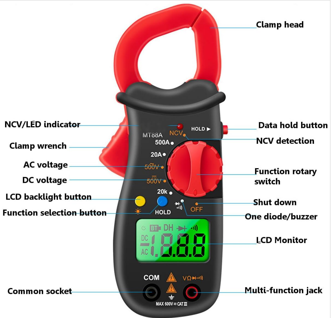
Figure 2.2: Detailed view of the MT88A Digital Clamp Meter with key components labeled for identification.
