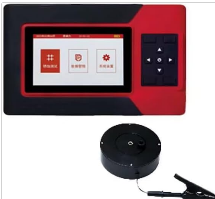
Figure 3.4: The main unit displayed with another sensor, possibly the potential electrode, essential for potential method measurements.
