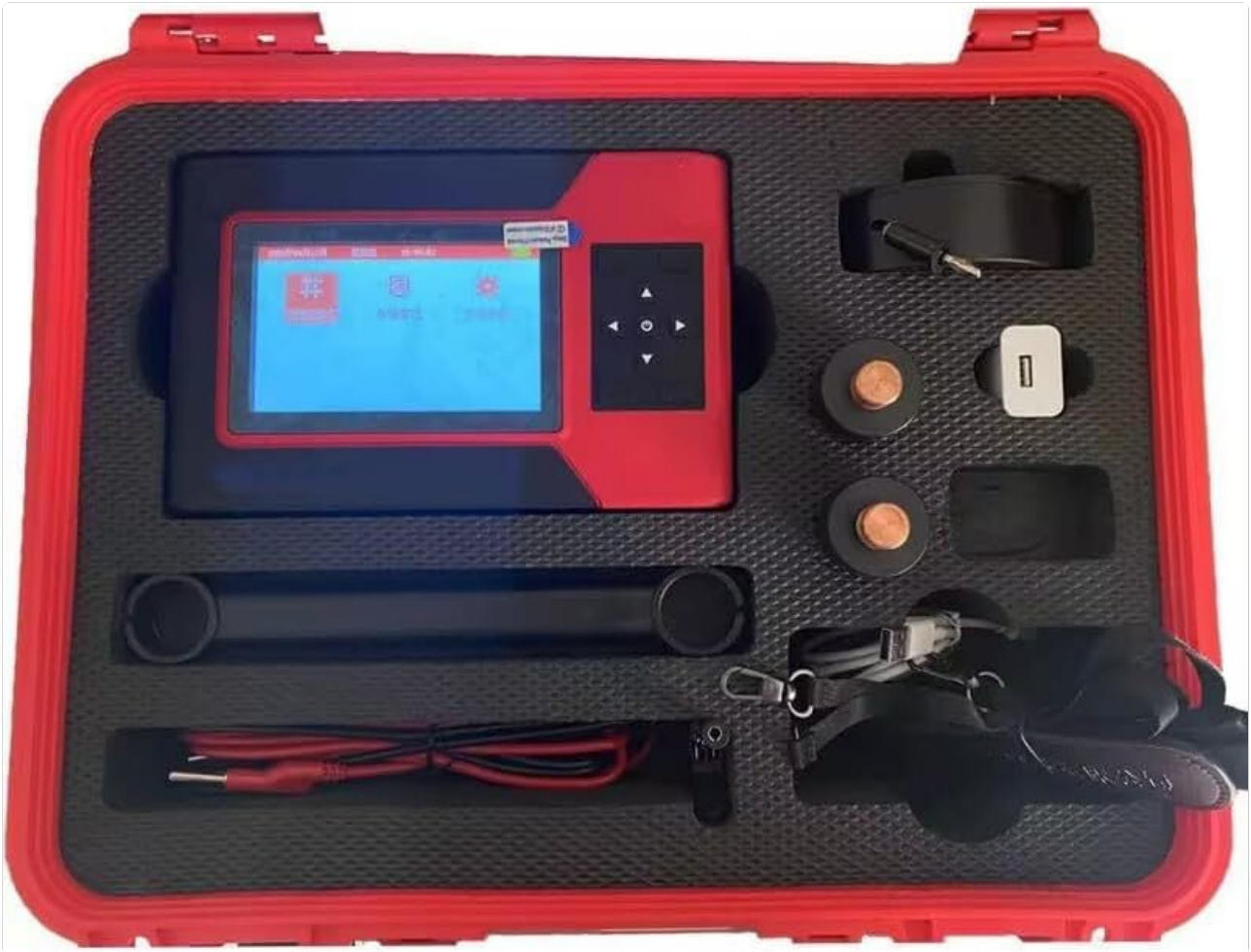
Figure 3.1: Complete set of the CNYST Rebar Corrosion Meter and its accessories, neatly organized within the protective red carrying case.
