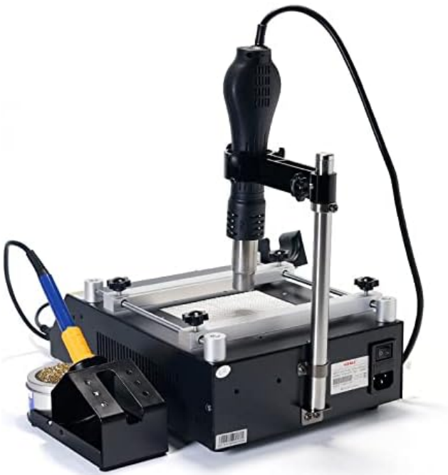
Figure 3.4: Side view of the 853AAA rework station, showing the power switch and power input on the rear panel.
