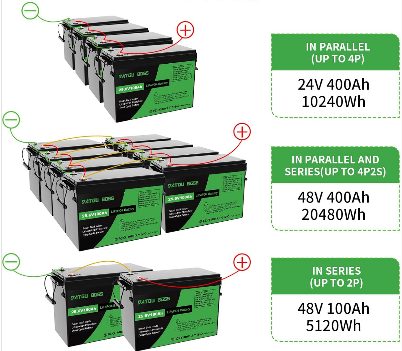
Image: A visual guide demonstrating how to connect multiple DATOU BOSS LiFePO4 batteries in parallel, series, or a combination of both to achieve desired voltage and capacity configurations, with examples of total power output.
