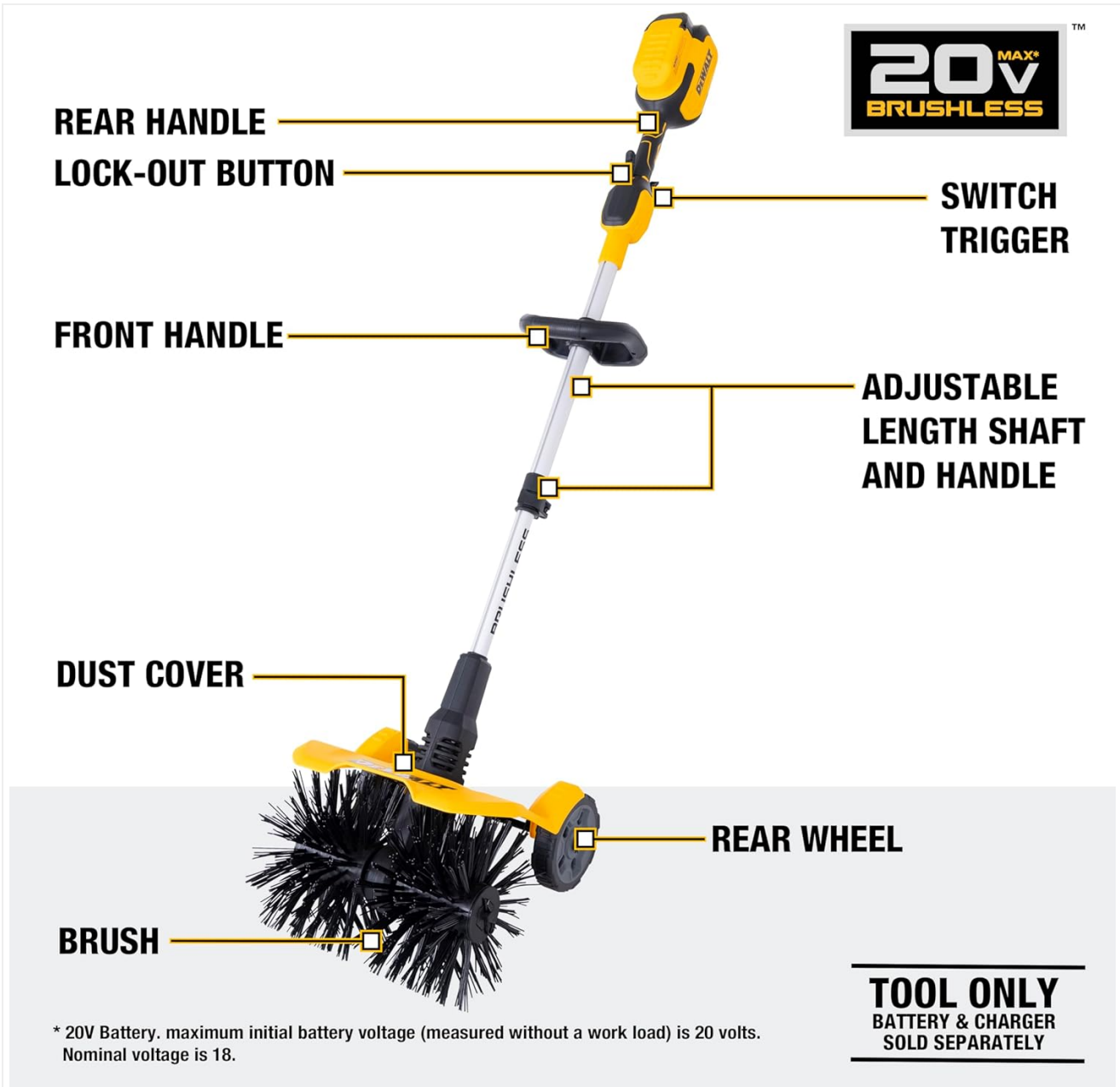
Figure 2: Labeled Components of the Sweeper Brush
