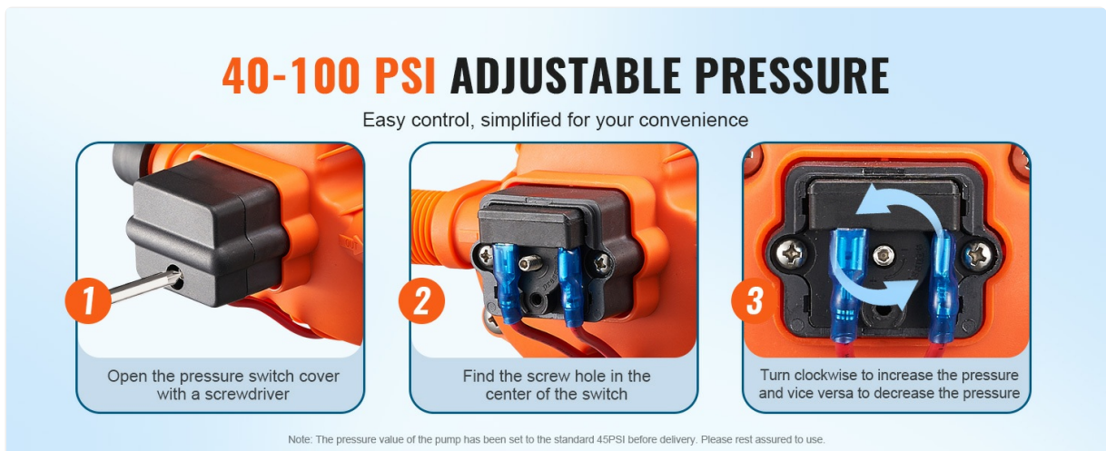
Image 6.1: Step-by-step guide for adjusting the pump's pressure switch.
