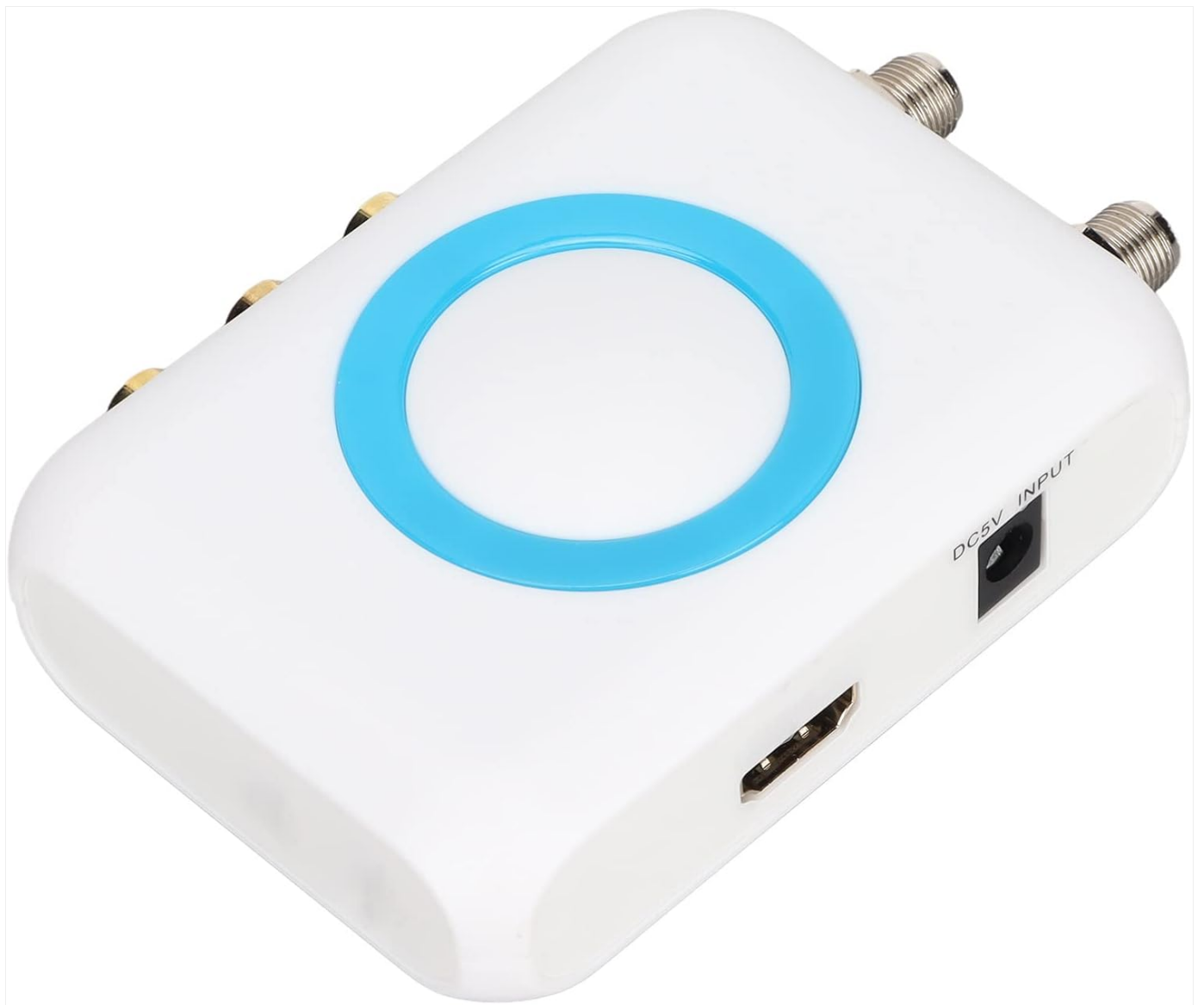
Figure 4.1: Rear view of the HDM66 HD Modulator, showing the DC 5V INPUT for power and the HD Multimedia Interface INPUT port.
