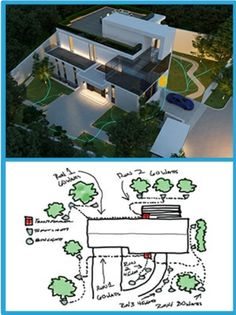
Image: An aerial view of a house with a proposed landscape lighting layout, accompanied by a hand-drawn diagram illustrating different lighting runs and their respective wattages, aiding in system planning.
