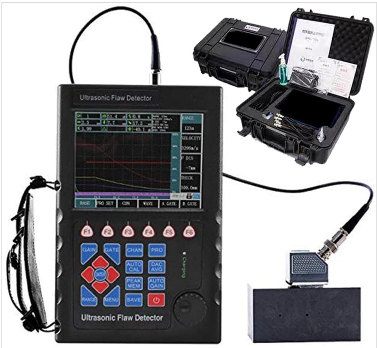
Figure 2.1: Ultrasonic Flaw Detector with its protective carrying case and essential accessories, including probes and cables.
