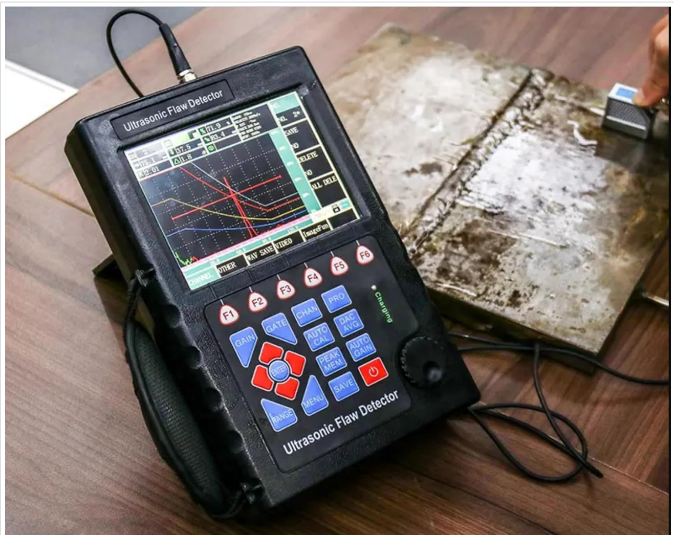
Figure 5.2: The Ultrasonic Flaw Detector actively performing an inspection on a metal workpiece, demonstrating its practical application.
