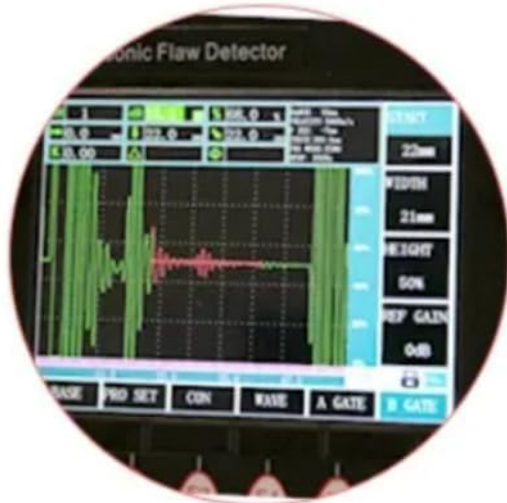
Figure 5.3: The device connected to a probe, illustrating its capability for various inspections including steel plate, casting, forging, and weld inspection.
