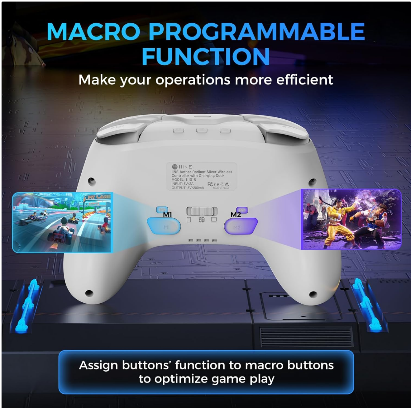
Image 4.1: The back of the controller showing the M1 and M2 macro buttons, which can be assigned functions to optimize gameplay.
