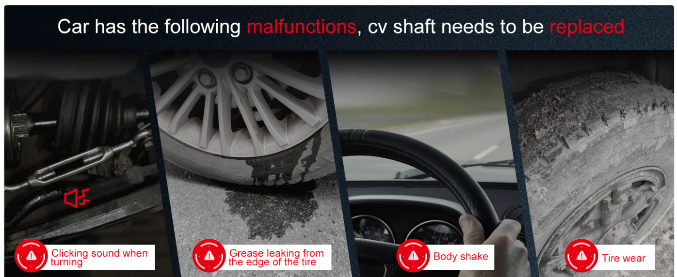
Figure 7: Visual guide to common signs of a failing CV axle, including clicking sounds, grease leaks, body shake, and tire wear.
