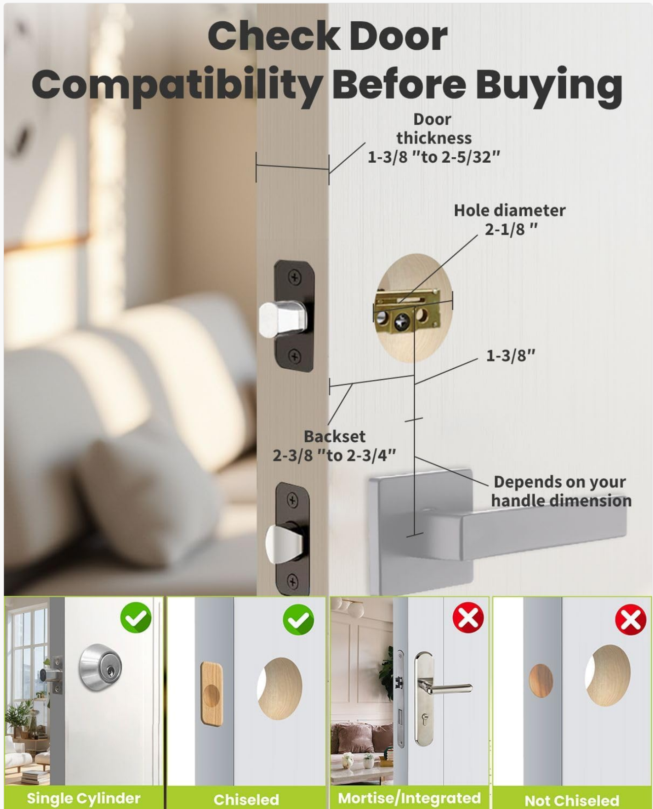
Image 3.1: Diagram illustrating door compatibility requirements for the UF03 Smart Lock, including door thickness, hole diameter, and backset measurements. It also shows compatible and incompatible door types.
