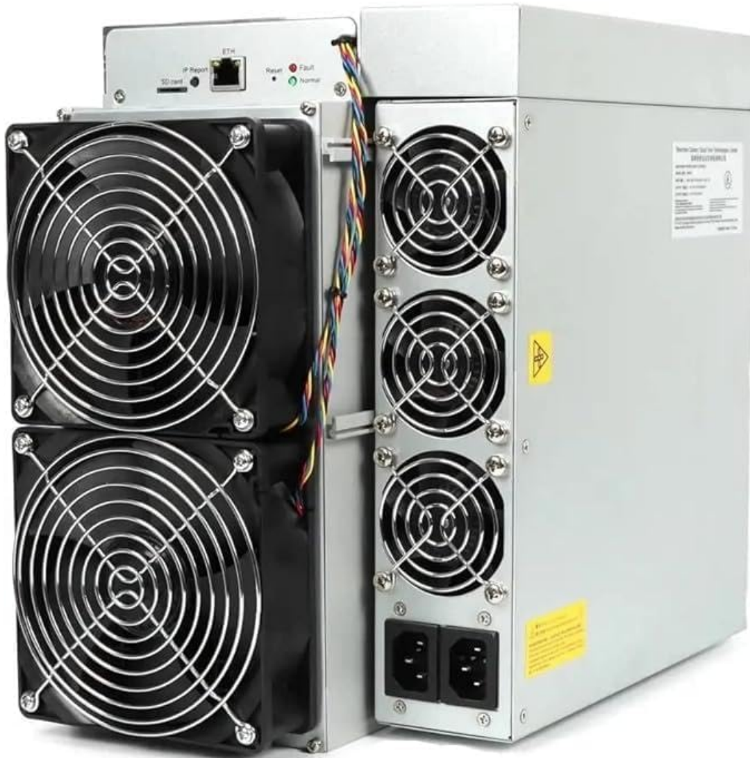
Figure 3: Rear view of the Antminer S19j Pro, detailing power connections and exhaust fans.
