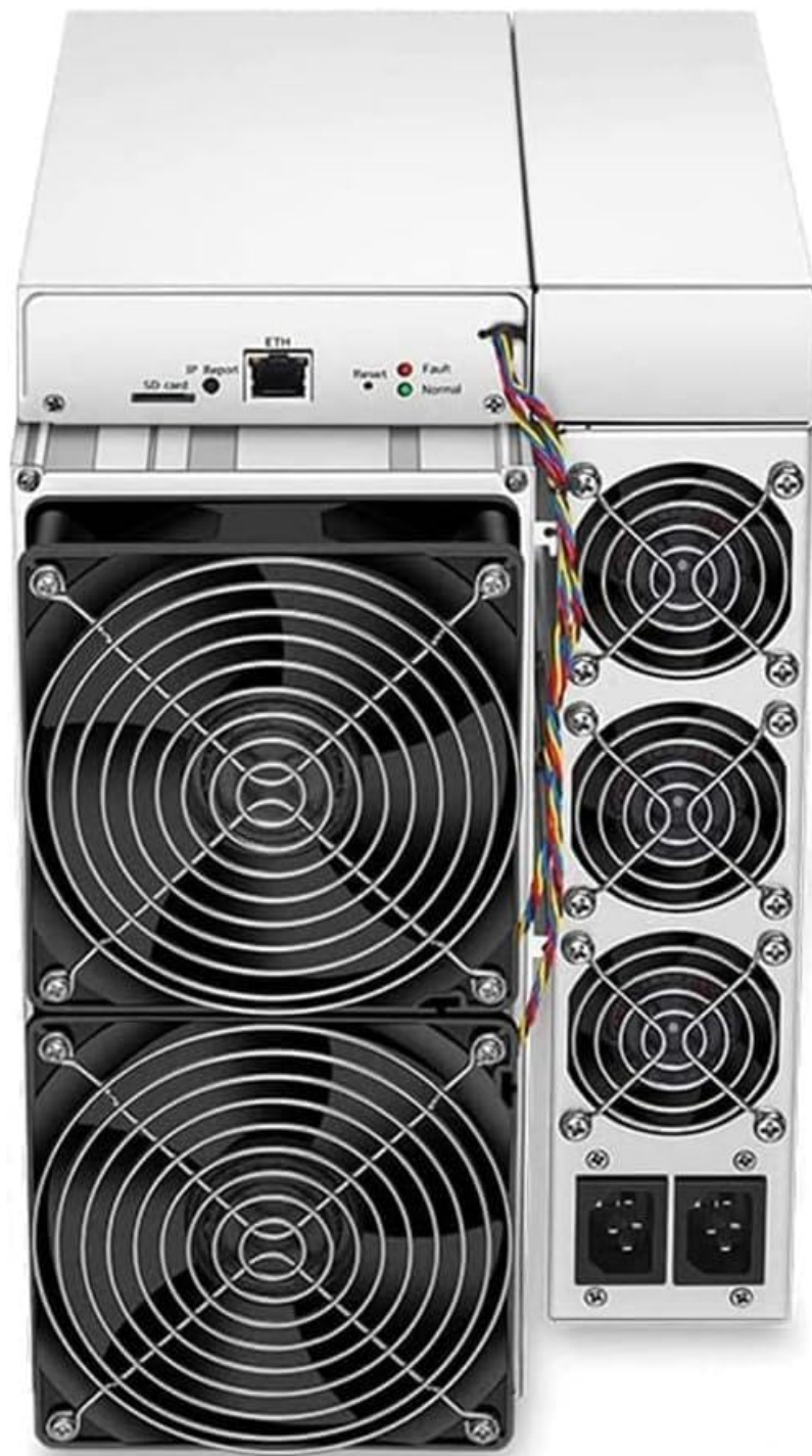
Figure 1: Front view of the Antminer S19j Pro, highlighting the control board and cooling fans.
