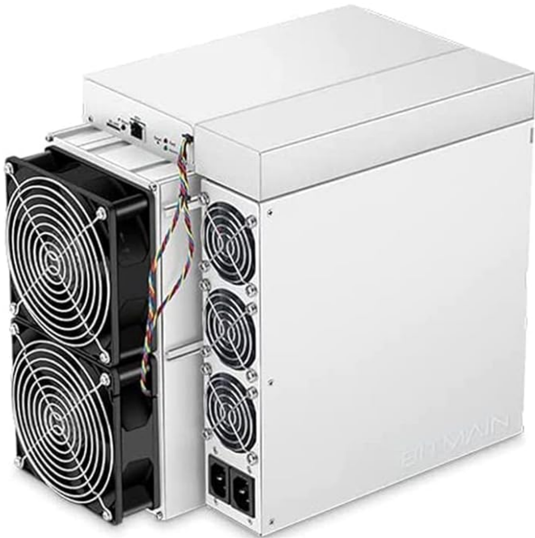
Figure 2: Angled view of the Antminer S19j Pro, showing both front and side cooling systems.
