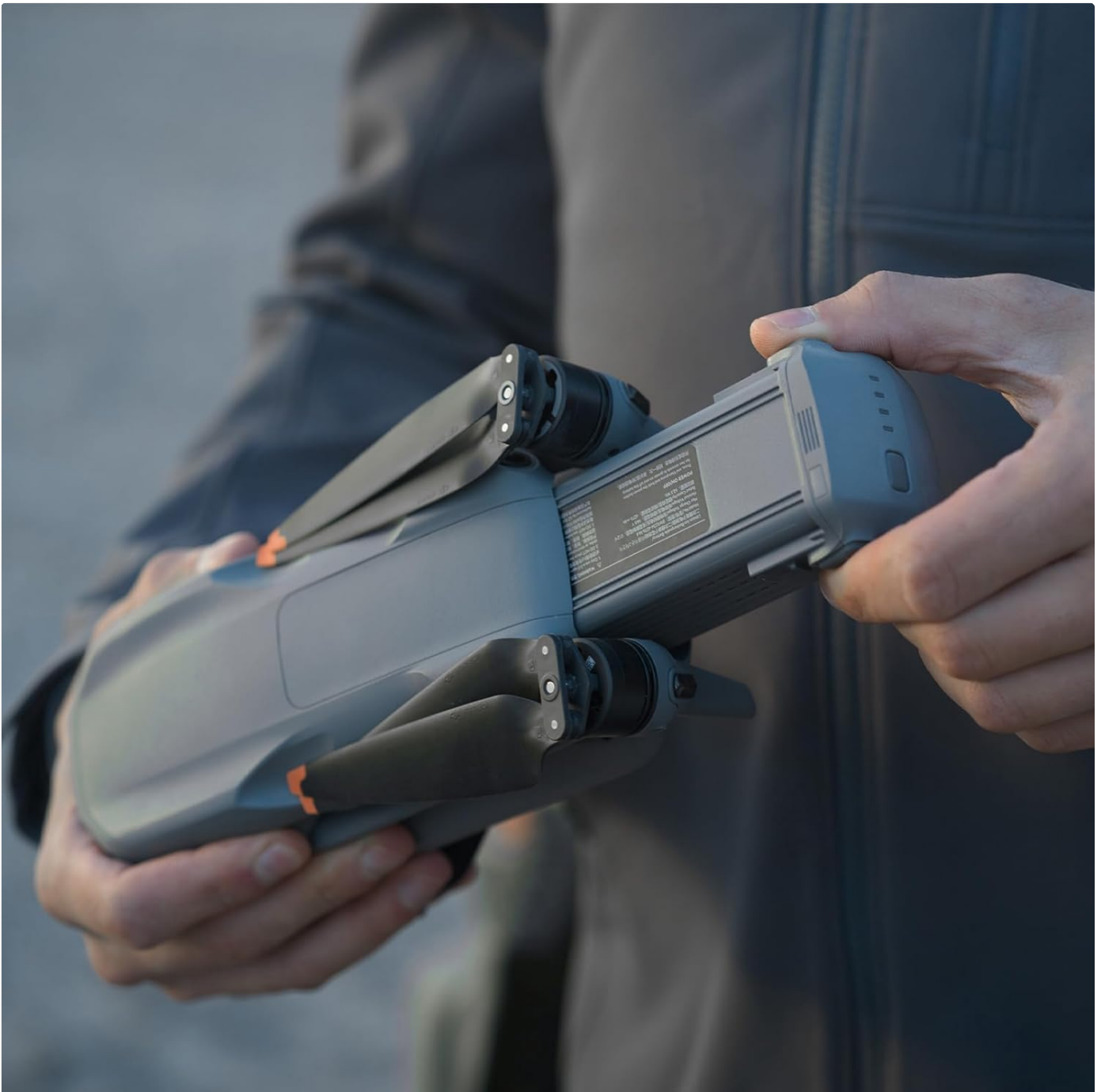
Figure 2: Proper installation of the Intelligent Flight Battery into the drone.
