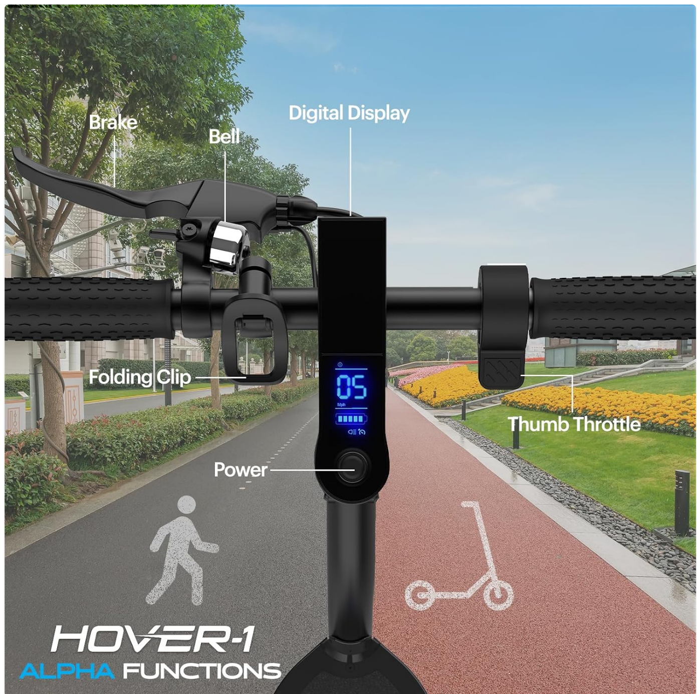
Figure 5: Overview of the scooter's controls and digital display.
