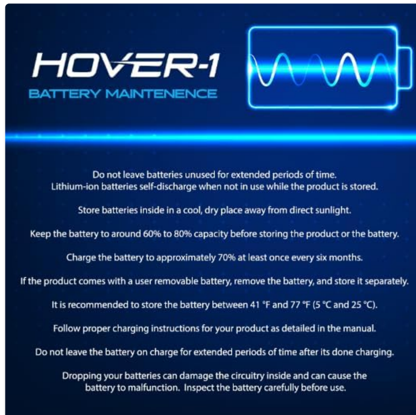
Figure 4: Important battery maintenance guidelines.
