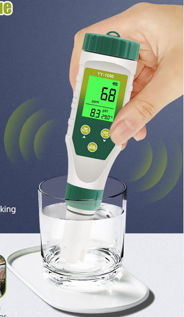
Figure 6: Checking the TDS value of drinking water. This image illustrates the tester's use for assessing the quality of tap water, bottled water, or spring water.
