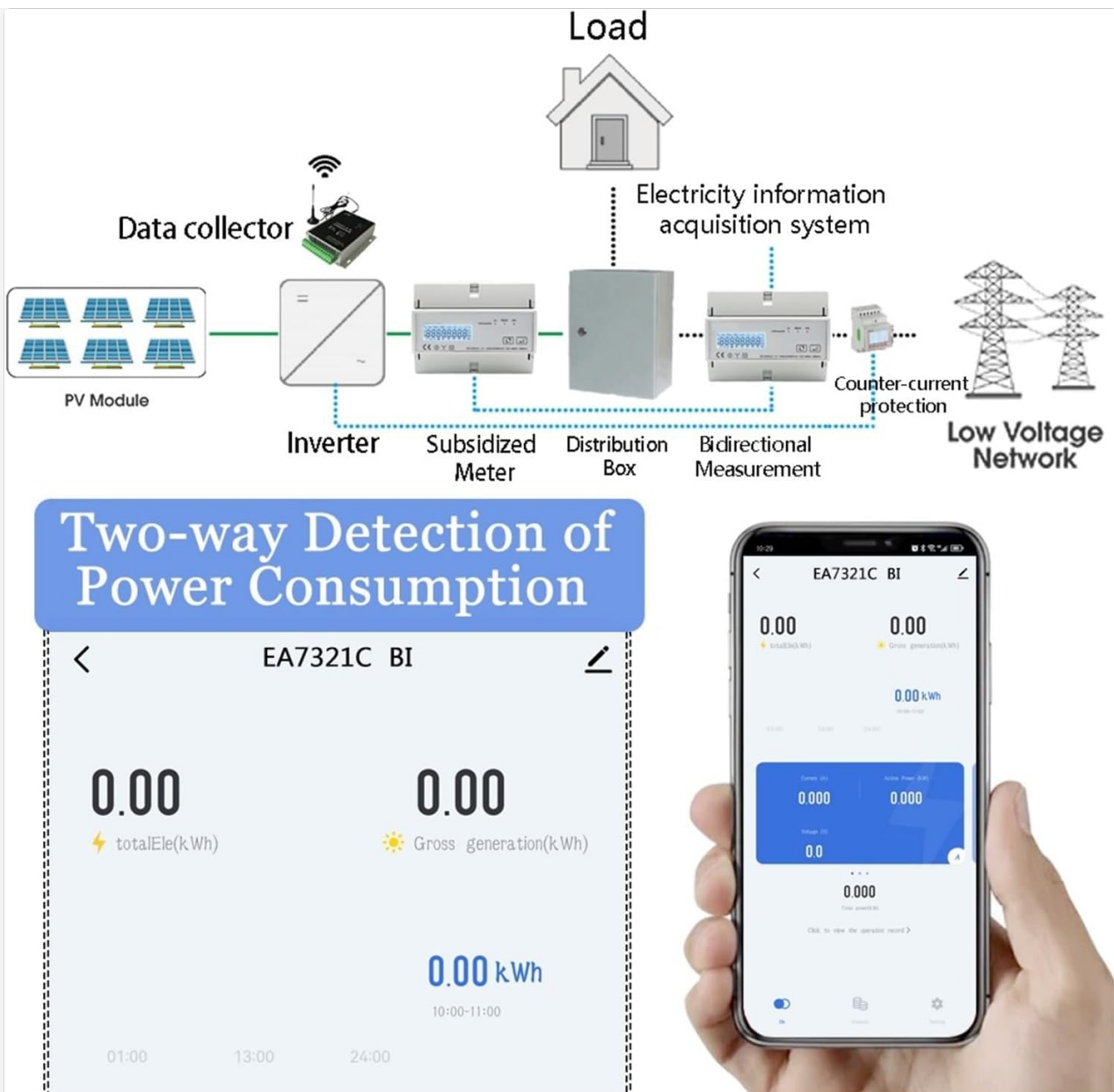
Image: A schematic diagram illustrating the two-way detection of power consumption, showing the flow from PV modules through an inverter, subsidized meter, distribution box, and bidirectional measurement to the low voltage network and load, along with a smartphone app interface displaying total energy and gross generation.
