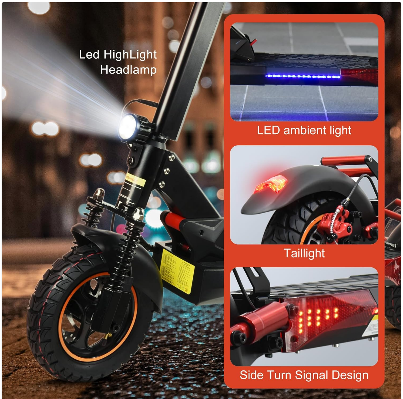
Figure 3.2.3: Overview of the scooter's lighting system, including the LED headlamp, ambient light, taillight, and side turn signals.
