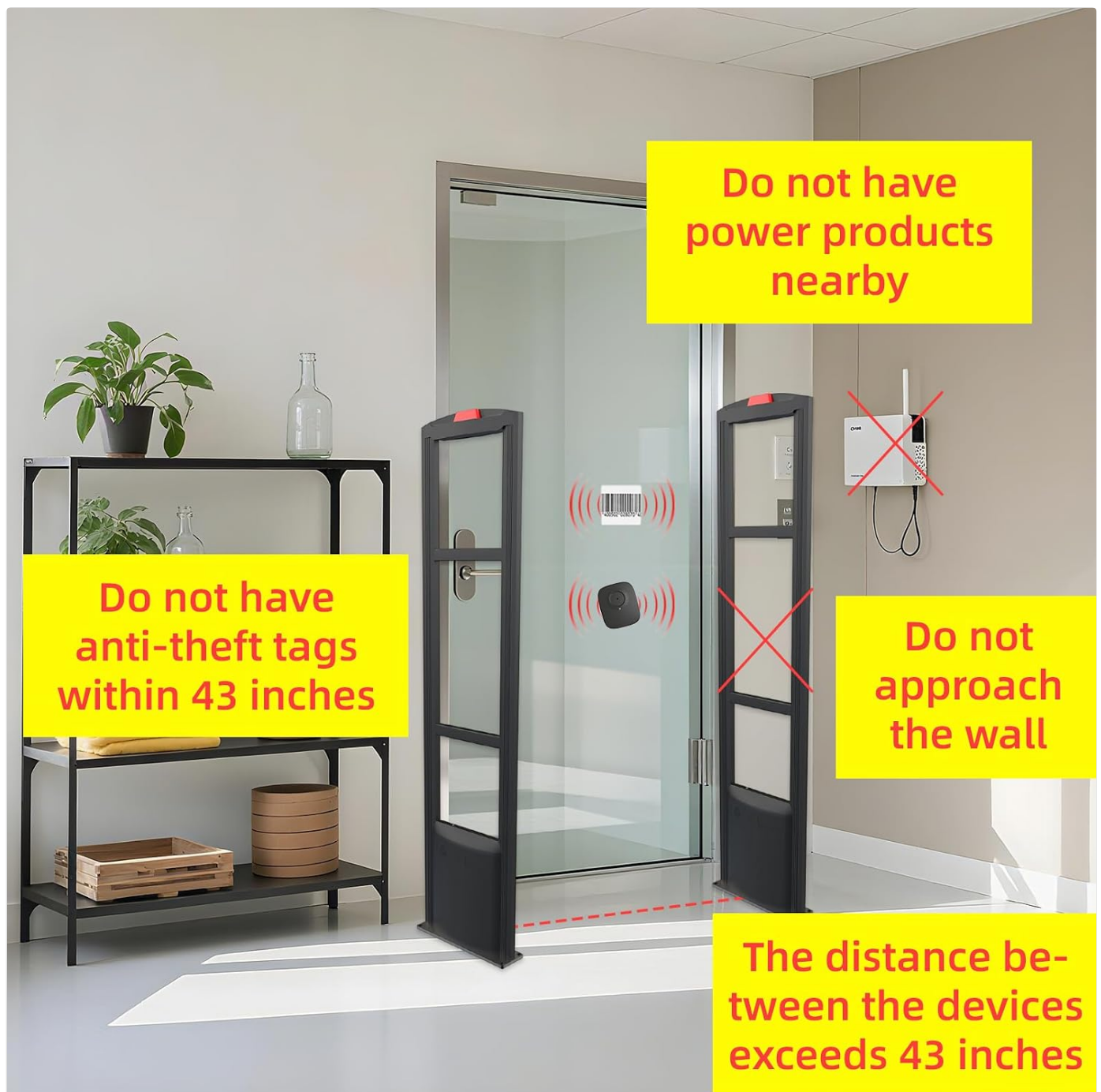
Figure 5.1: System Placement Guidelines
