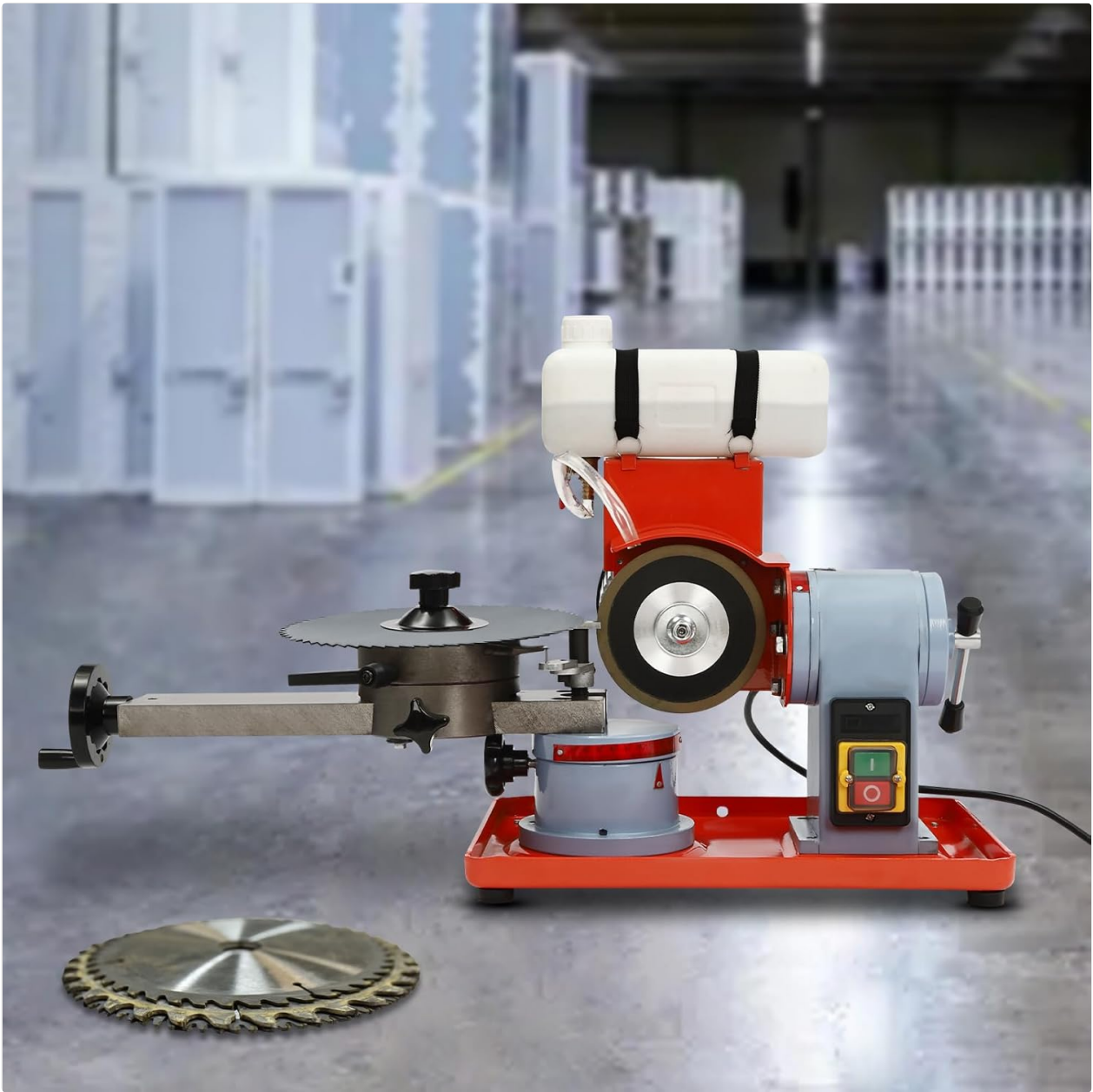
Figure 5.1: The saw blade sharpener in operation, demonstrating a circular saw blade mounted and positioned for sharpening.
