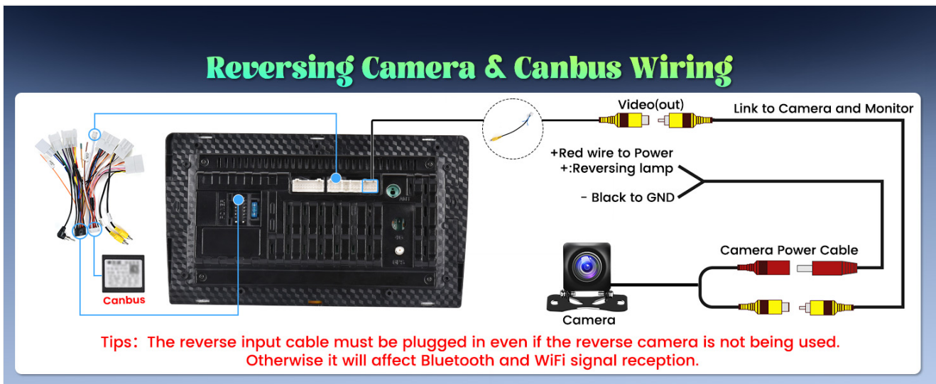
Image: A detailed diagram illustrating the connections for the reversing camera, including power, ground, and video input, as well as the Canbus wiring.
