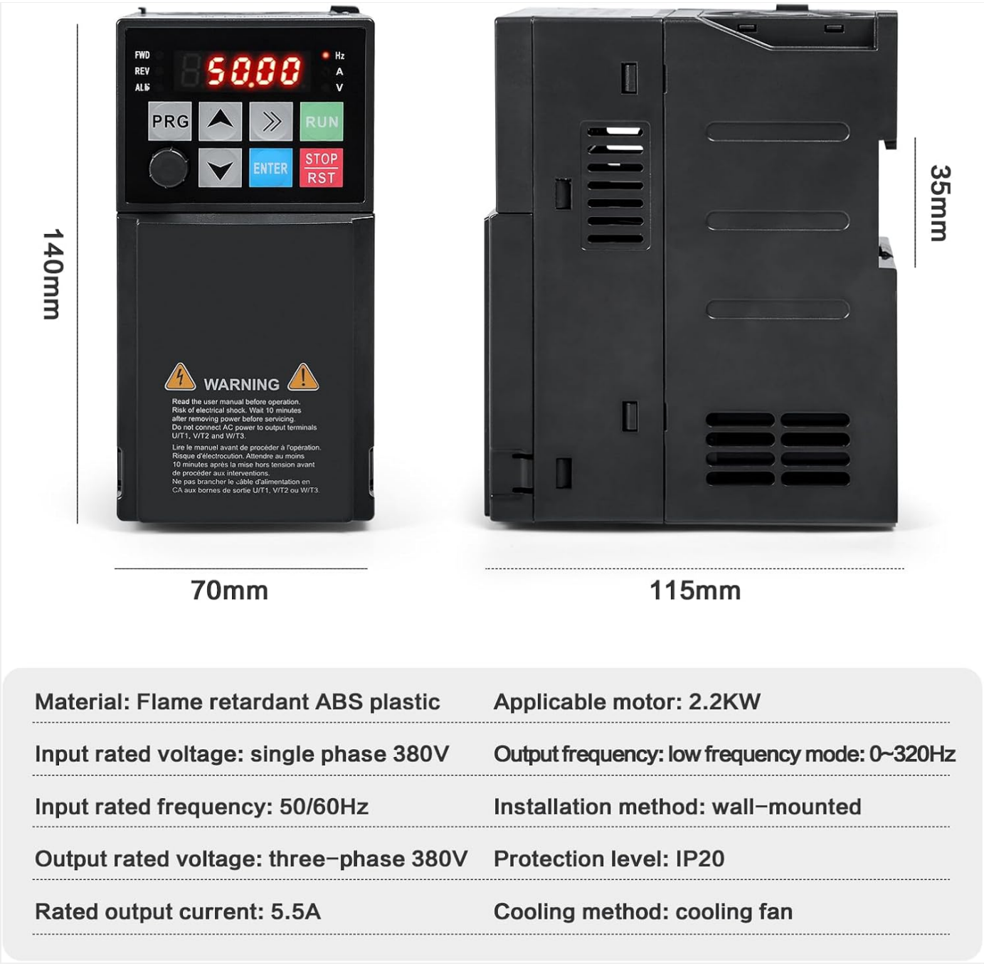
Figure 3.2: Diagram illustrating the dimensions of the Telituny Frequency Inverter (140mm height, 70mm width, 115mm depth, 35mm panel depth) and a table of key specifications.
