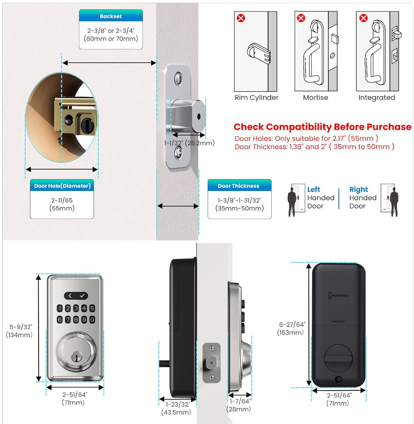
Image: Door compatibility diagram. This image illustrates the required door dimensions and incompatible lock types for the S11A model.
