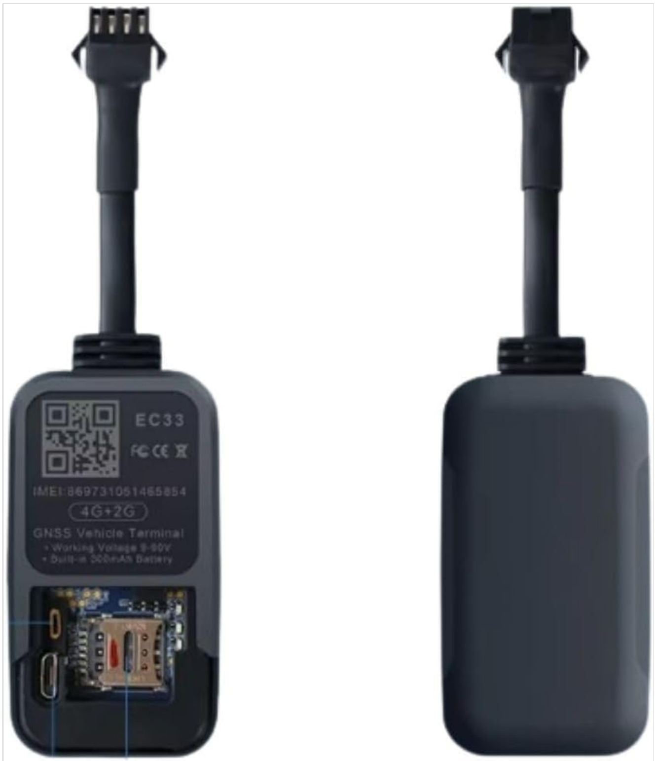
Figure 2: Front view of the Genérico EC33 Vehicle Tracker with the cover removed, revealing the micro SIM card slot and Type-C data port. This image shows the internal components for SIM card insertion.
