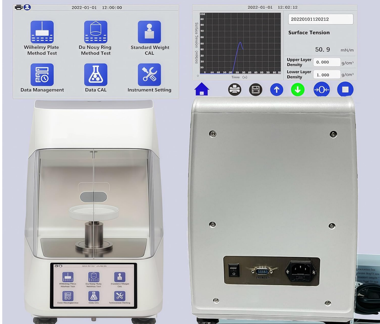
Figure 4: The user-friendly test interface of the VTSYIQI AITS-800P, displaying real-time surface tension values and a dynamic measurement curve.
