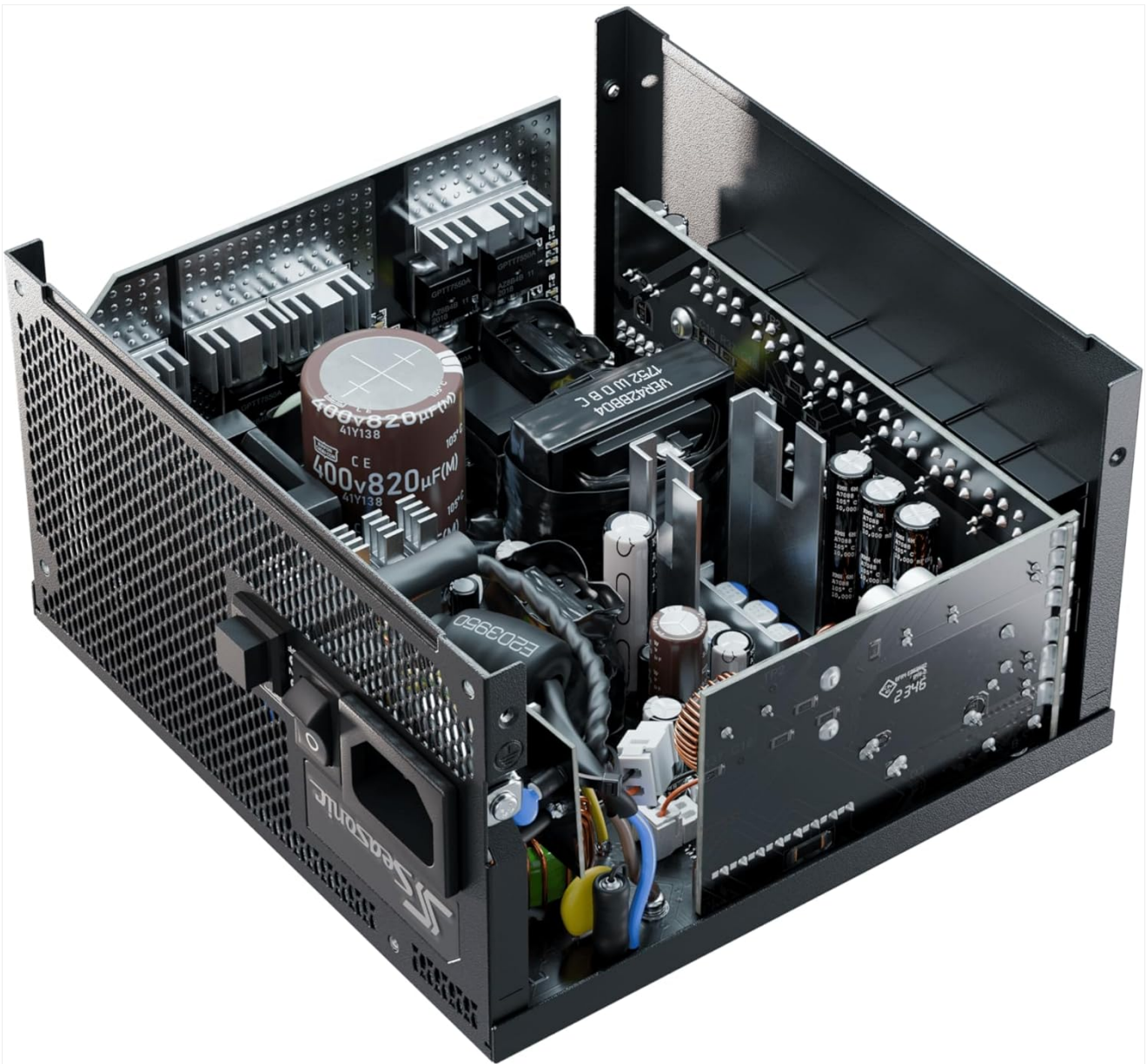
Image: An internal view of the Seasonic Focus V4 GX-1000 power supply, illustrating the high-quality components and efficient layout that contribute to its performance and reliability.
