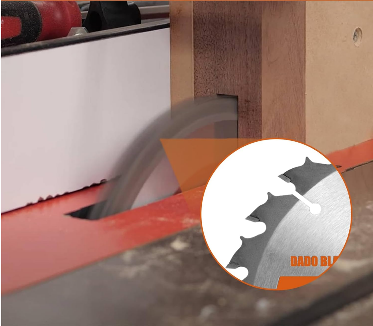
Image 6.1: Example of the dado blade in operation, creating a clean groove.
