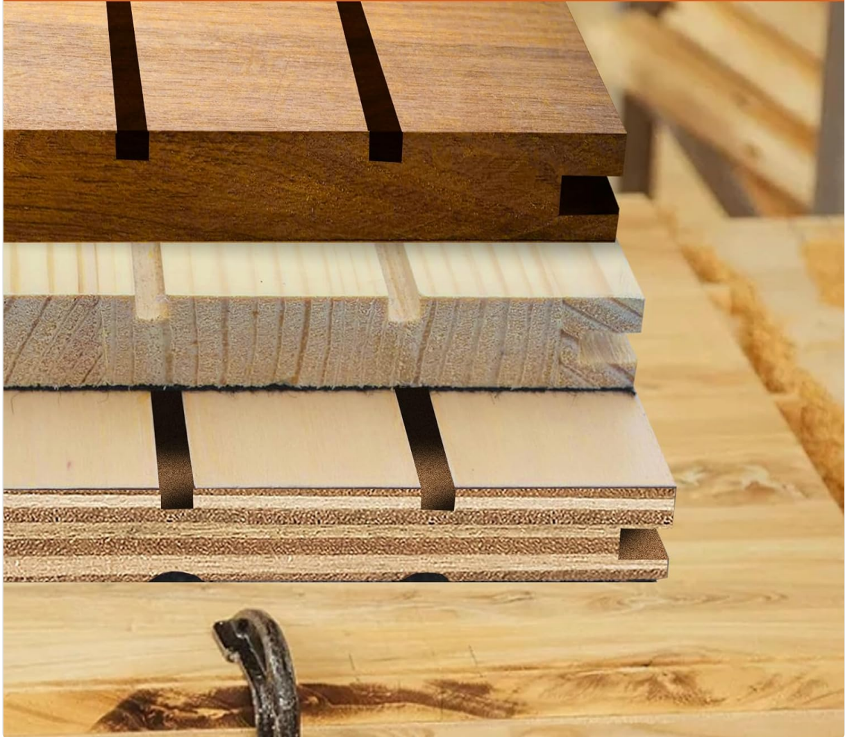
Image 6.2: Examples of various dado cuts in different wood types, showcasing versatility.
