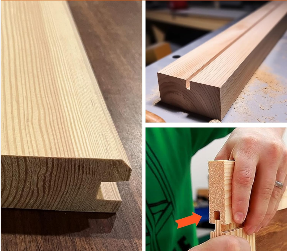
Image 6.3: Detailed views of precision cuts and joint assembly using the dado blade set.
