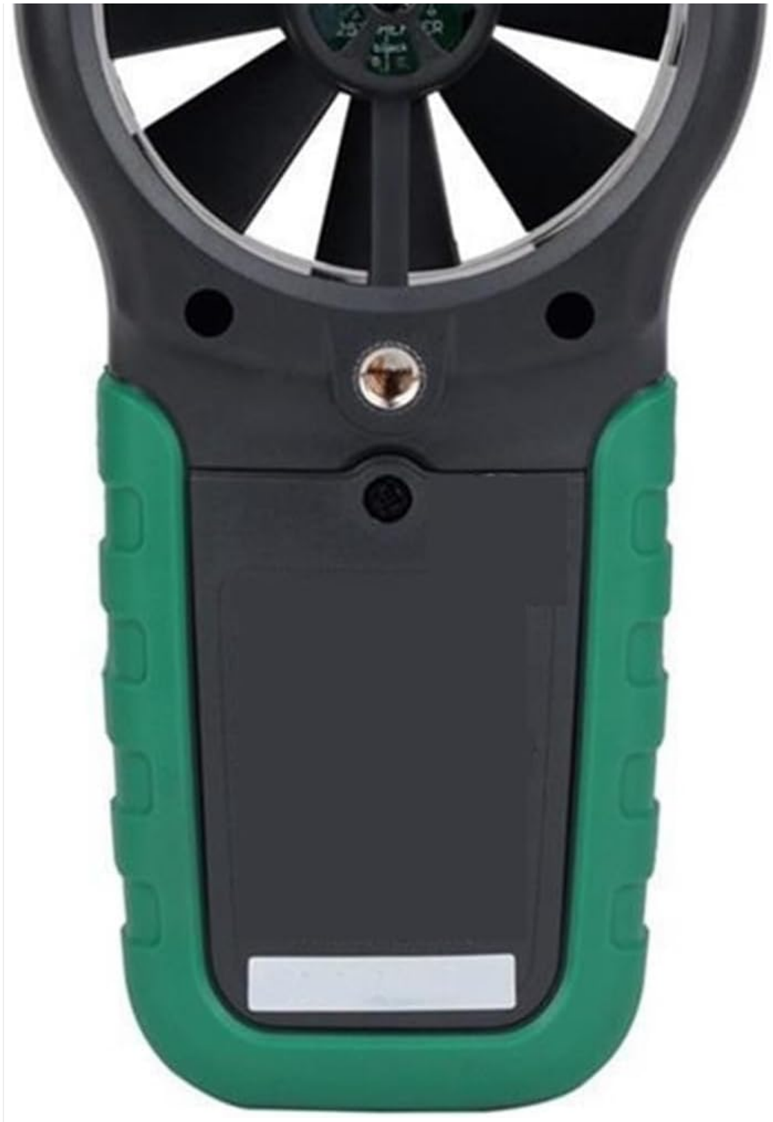
Figure 2: Back view of the MS6252A Anemometer. This image shows the rear casing, which typically houses the battery compartment and may include a tripod mounting screw hole.
