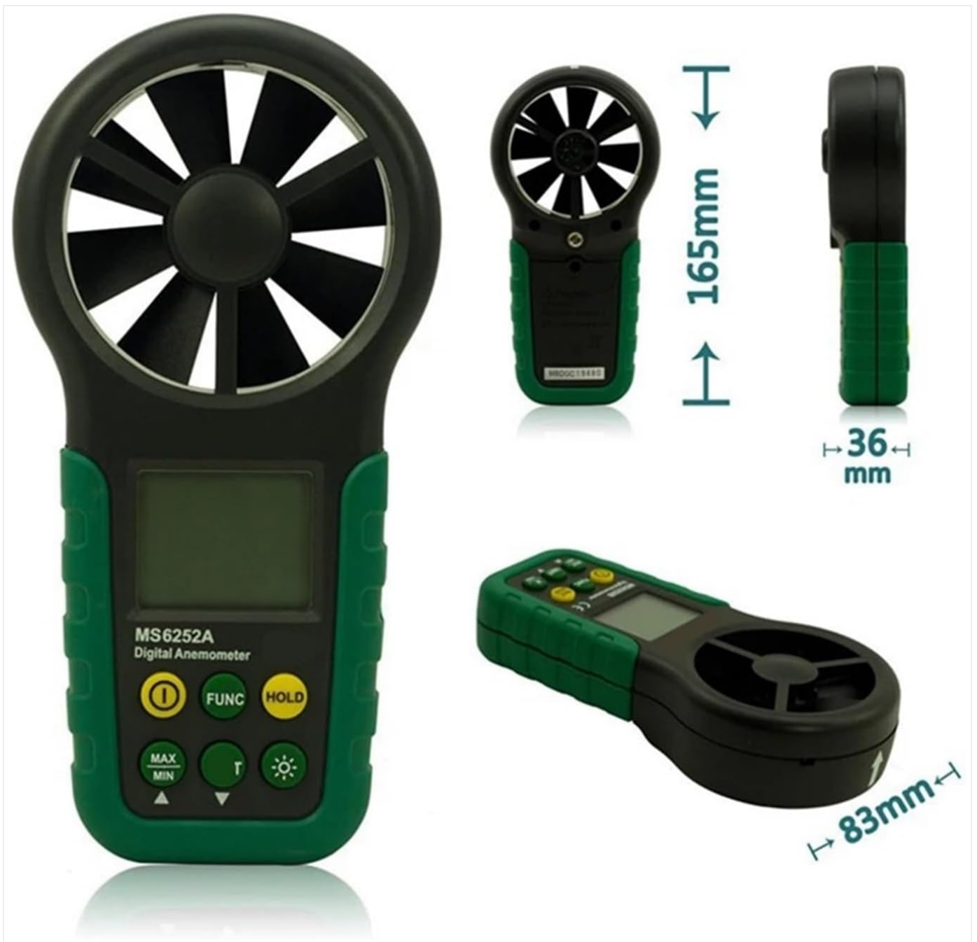
Figure 1: Front and side views of the MS6252A Anemometer. This image illustrates the device's overall design, including the impeller, digital display, control buttons (FUNC, HOLD, MAX/MIN, backlight), and approximate dimensions (165mm height, 83mm width, 36mm depth).
