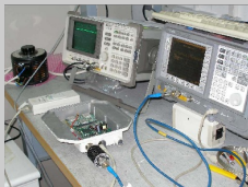
Test setup : CPE ODU radiated
