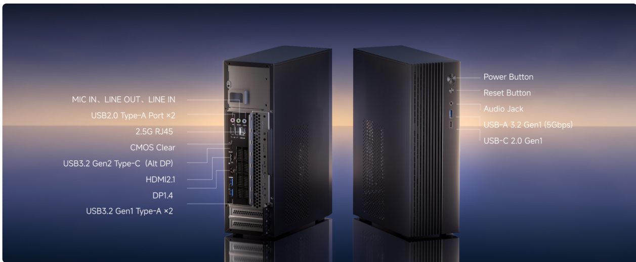
Image: A detailed diagram showing the front and rear I/O ports of the MINISFORUM 795S7 for connecting peripherals.
