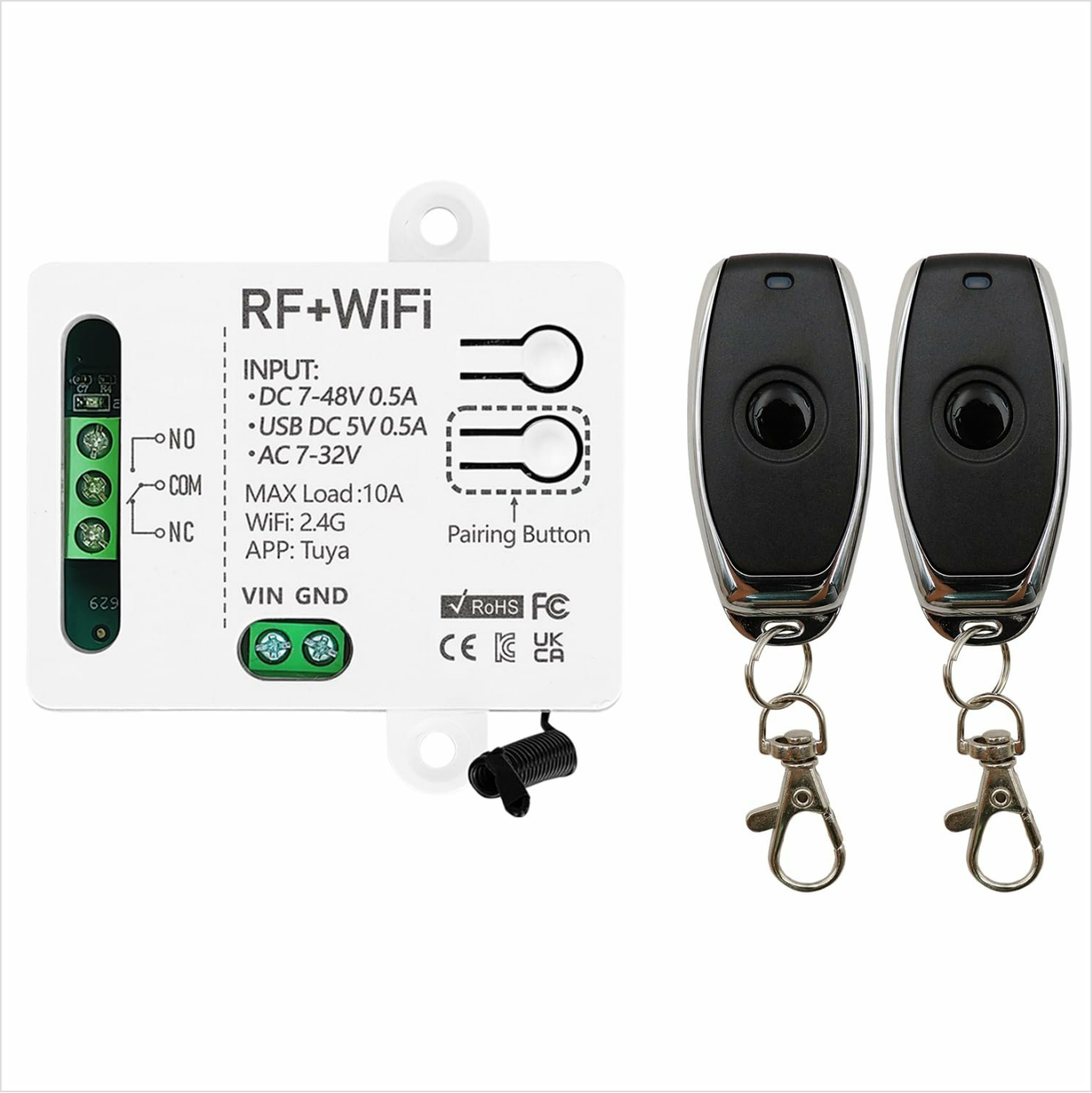
Figure 4.1: The smart switch module and the two accompanying RF remote controls.
