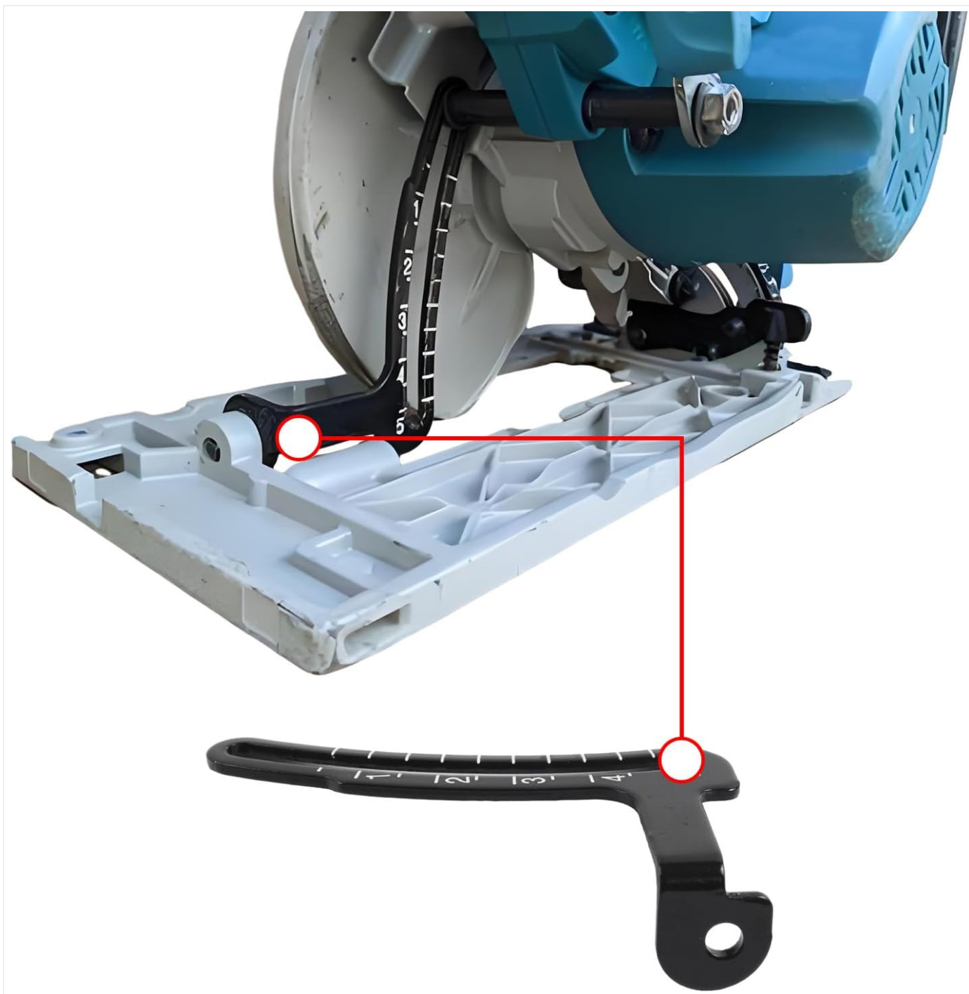
Figure 2: Illustration showing the depth guide being installed into the base plate of a circular saw. The red line indicates the alignment point.
