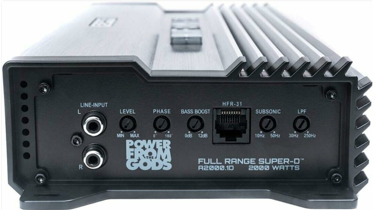
Image: Rear panel of the Hifonics Alpha A2000.1D amplifier, displaying the Line-Input (RCA), Level, Phase, Bass Boost, HFR-31 remote port, Subsonic filter, and LPF (Low-Pass Filter) controls.
