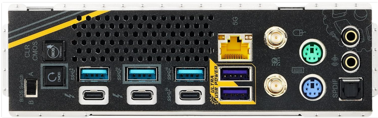
Figure 4.1: The rear input/output panel, showing various ports including USB, Thunderbolt 4 Type-C, Ethernet, and audio jacks.
