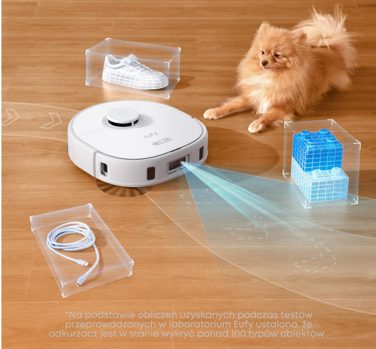
Image 5.4: The AI.See technology enables the robot to recognize and avoid common household obstacles.
