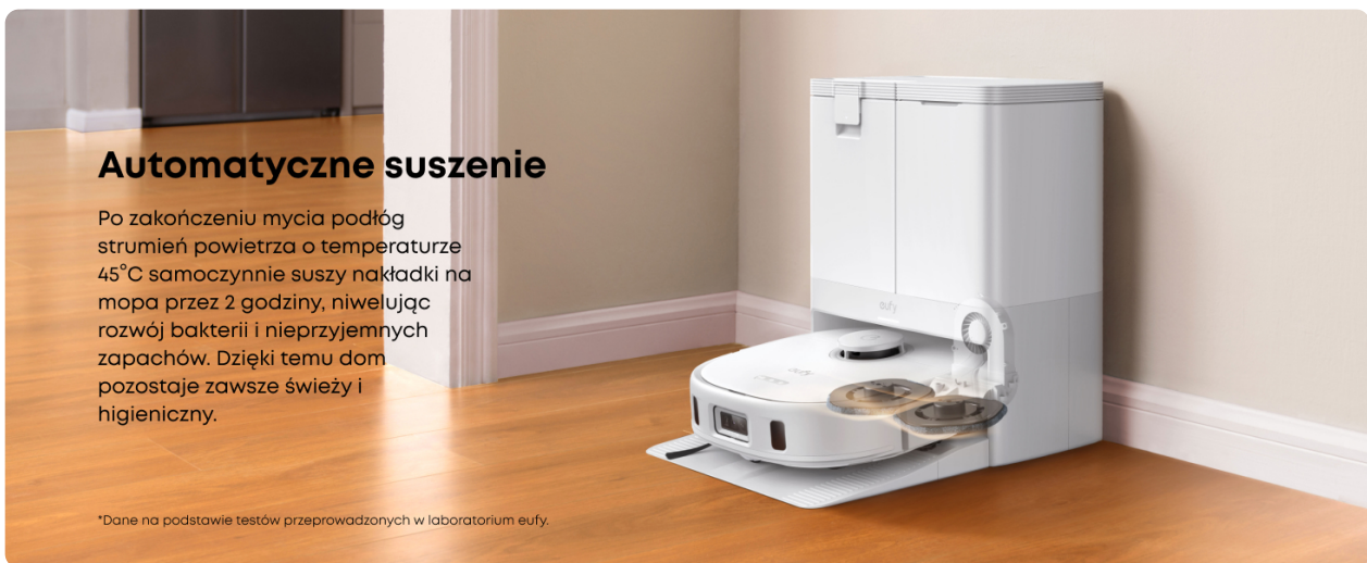
Image 6.3: Mop pads are automatically dried with 45°C warm air to prevent odors and bacterial growth.
