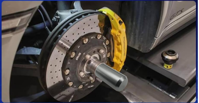
Image: The ZKTOOL alignment tool inserted into a vehicle's center lock hub, demonstrating its use as a guide during wheel removal or installation.
