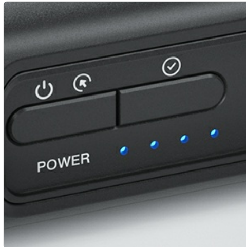
Figure 5: Close-up of the power button and LED indicator lights, showing the battery status.
