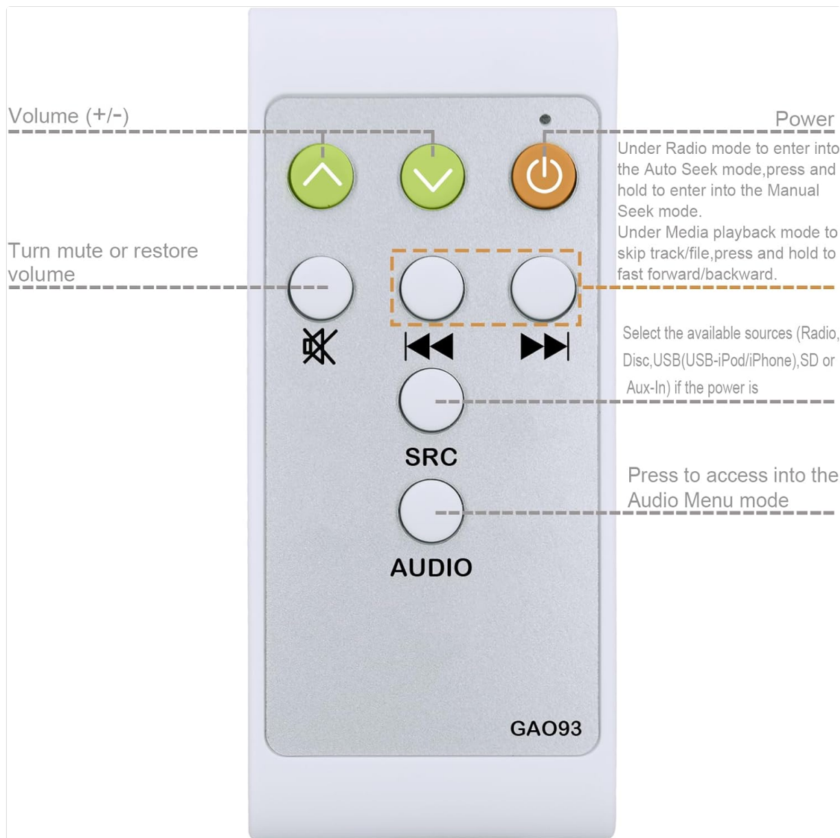
Image: Detailed diagram of the remote control buttons with their corresponding functions labeled.
