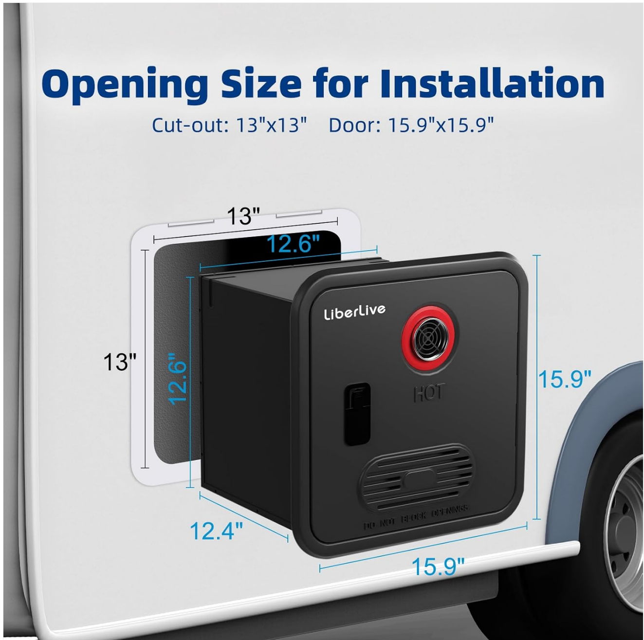
Figure 3: Installation dimensions for the water heater.
