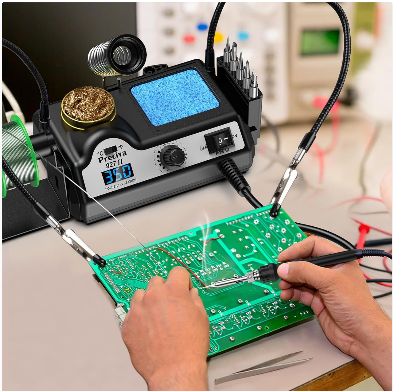
Image: A user actively soldering a circuit board, demonstrating the use of the helping hands.
