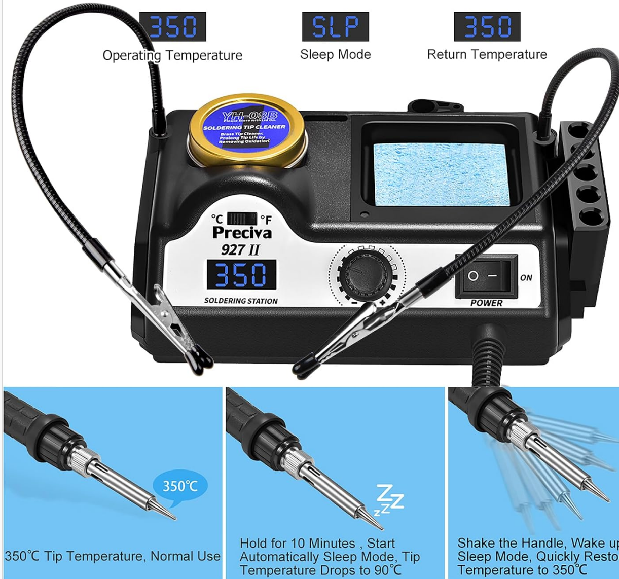
Image: Illustration of the 10-minute auto-sleep mode and wake-up function.
